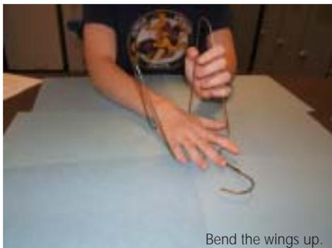
1) Bend both wings up so the catapult stands upright. The wings become two vertical and parallel triangles. Sometimes the coat-hanger is easier to bend if you place your foot or hand in its center and pull the coat hanger up around it.
